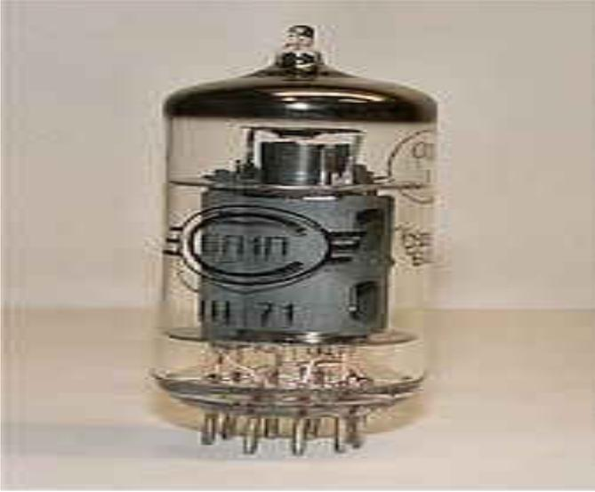
Murray Hill, New Jersey, were working to discover a device to replace the present vacuum tube technology. Vacuum tubes were the only technology available at the time to amplify signals or serve as switching devices in electronics. The problem was that they were expensive, consumed a lot of power, gave off too much heat, and were unreliable, causing a great deal of maintenance.
